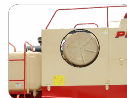
Bigger shields covering rotated parts with extra safety & Engine cooling by clean air through rotating sieve
