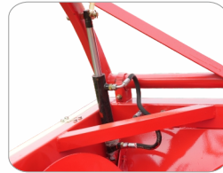
Jack Mechanism on the Reel Offers Extra Lifting strength
