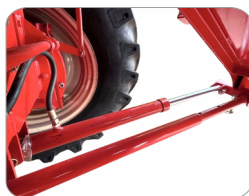
Hydraulic Jack With Independent Mechanical Supports
