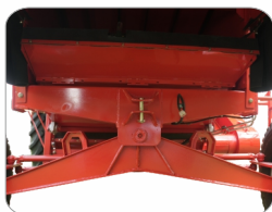
Rear Axle Mounting With Long Support Brackets
