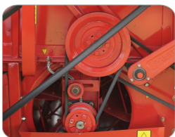
Pulleys With Coupling Mechanism
