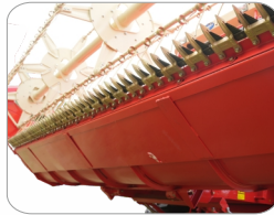
Cutter Bar Frame With Extra Supports
